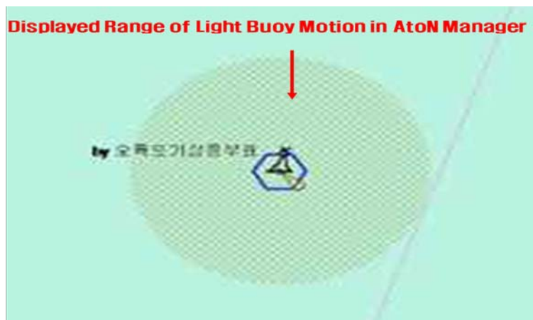
Figure 7: Light buoy motion result by wind and tidal current (2D screen)
