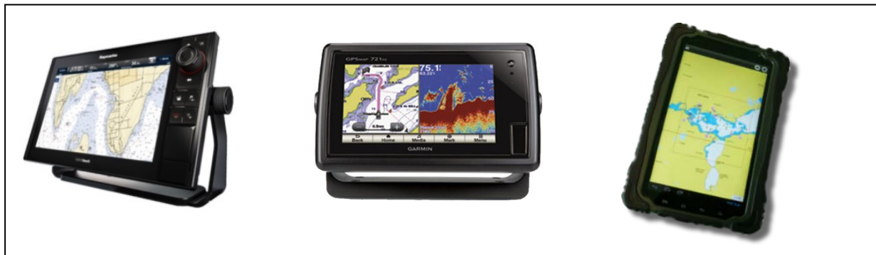
Figure 1: Three ECS types for pleasure crafts as used in the first study.
