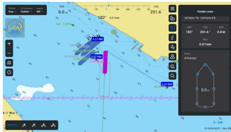
Figure 2, Example of Distance Measurement Function on Mapsea Navigation
