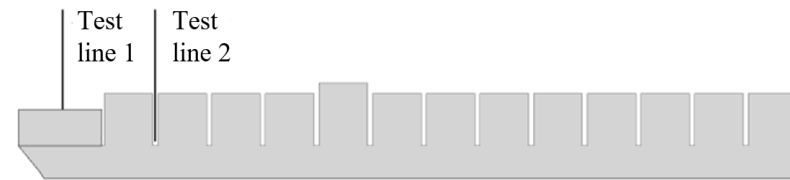
Figure 5. Monitoring line position for the ship with polygonal arcuate fairing
